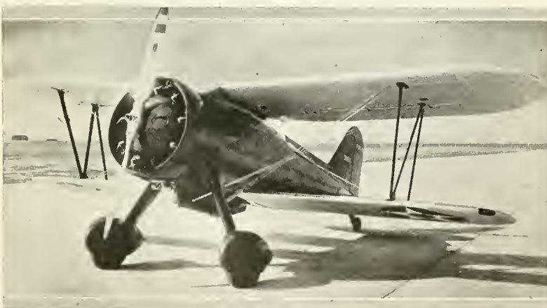
Curtiss F9C-2, Navy's newest and smallest airplane, to be carried by the "Akron"
